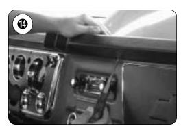
The Phillips head screws above the radio will pull the center of the pad tightly against the metal. You will see the dimples where the screws will push through and find the factory holes.
