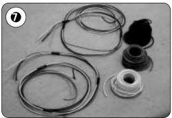
Purchase three rolls of different colored wire to make individual harnesses for each gauge. Yellow (lights), red (power) and black (ground) will work and allow you to differentiate as to the use of each wire. There will also be a sending unit wire or cable, so follow the gauge installation instructions for this connection.
