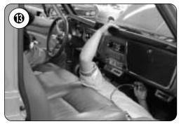
Once the dash is in place and the wiring routed, start installing the washers and nuts at each corner and the two screws above the radio. This will hold the pad securely. A few heavy books along the front edge will help the cement to bind to the metal dash.
