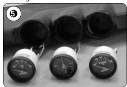
The gauges are positioned in front of the selected pod waiting for the wiring. It's advisable to pick your gauges and their position carefully, as you don't want to have to remove the pad in the future because you made a wrong decision at this point.
