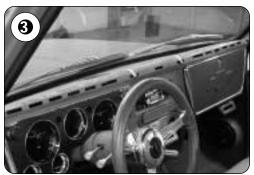
Here's the original metal dash with the factory pad removed. There will be four new attaching points for the gauge pad, one at each corner and two in the middle above the radio. These are original factory provided holes, so no drilling is necessary. The studs and holes in the new pad will match up to the originals.
