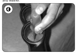
Begin by punching a hole with an awl or screwdriver through the foam in the back of each gauge pod. This will allow the wiring to be pushed through the foam and be connected to the rear of each gauge. A quarter inch diameter hole will work nicely.
