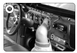
With the pad resting on the dash, feed the wire harness through the existing hole in the dash along with any sending unit tubing or cables, and route them over the radio toward the fuse box. This will enable you to reach that power source if needed and feed sending unit connections through the firewall.
