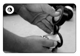
If the gauge fits slightly loose in the pod, wrap electrical tape around the housing behind the bezel until it fits snugly. You don't want it to be too tight or you won't be able to turn it once the pad is installed. A snug fit will still allow you to pull it forward in the future if necessary.
