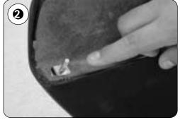
There is a stud installed at each corner of your new dash pad that corresponds to a factory hole used to mount the original pad. Attaching hardware for these studs is included. You must reach up under each corner of the dash once the pad is in position and install and tighten the supplied 3/8-inch nut and washer.
