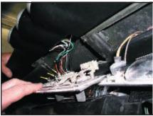
15. With the Maxipad again trial fitted, we notice another possible problem: The heater controls' moving studs tended to snag on the new gauge wiring
