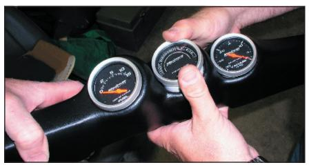
4. Three standard 2-1/16" gauges, of any brand or type you lust after, slide right into the gauge holes, held firmly in place by friction.
