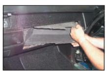
5. The old pad comes right out. Right. Make that, it comes right out after you remove the mounting nuts, which are buried deep in the bowels if the dash structure. Access isn't easy; begin by removing the glove box.
