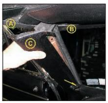
6. Both A-pillar trim panels (c) must be removed, along with the windshield header trim panel (b). It's just a few Philips screws. You'll also need to remove at least the front screw from the roof rail inside trim panel (a) because it traps the A-pillar trim panel.
