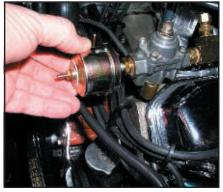
17. Hook up the gauges per the manufacturer's instructions, and install any senders required (here, a fuel pressure transducer is going in). Remember that lighting wiring should be connected to a stock orange variable-voltage (i.e., dimmable) wire on the stock cluster. Now simply reverse steps 92 thru 1 to bolt it all back together, and enjoy your new information sources. And the enviable glances the super-cool appearances will provide.
