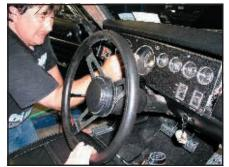
7. You'll also need to lower the steering column to remove the entire stock cluster. Try not to grimace while doing this. Also drop the heater control panel (but do not disconnect it.) Again, all of these shenanigans is required just to get to...
